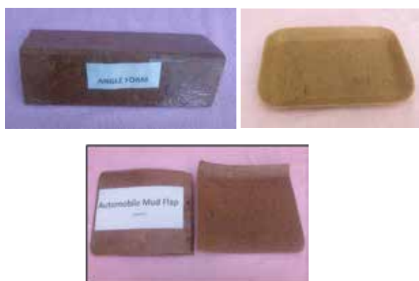
Products developed using polylactic acid and coir composites
