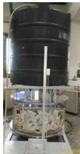
Drying and pressure drop determination in 1 m diameter pile with dead weight for compression
