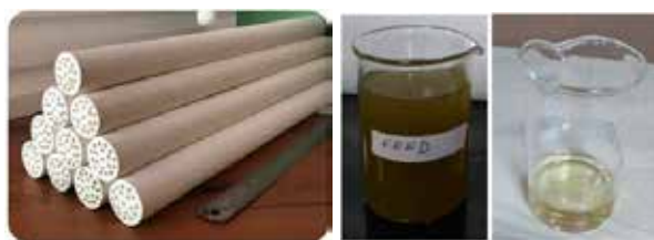
Multi-channelled ceramic membrane tubes (left) and sugarcane juice clarification through the developed membranes
