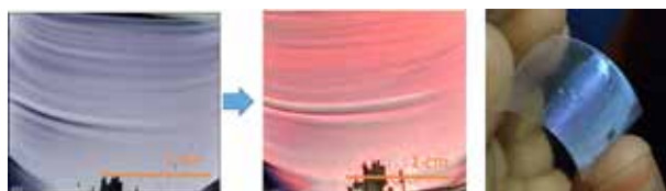
Angle-dependent color changing photonic crystals on solid and flexible surfaces
