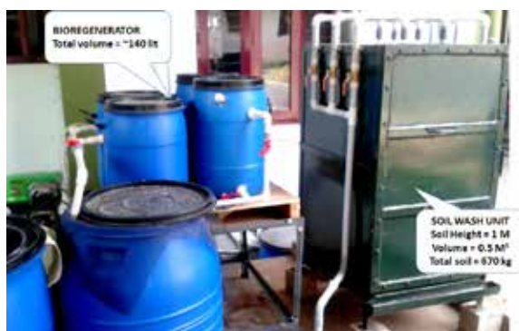
Pilot plant unit (670 kg/batch) for demonstrating perchlorate contaminated soil remediation.
