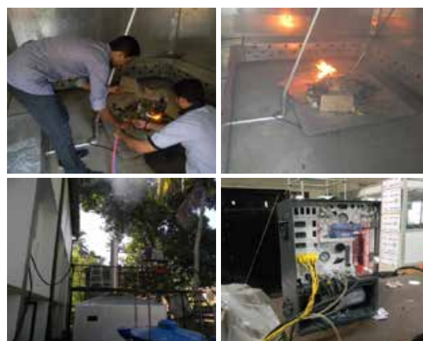
Simulated waste combustion experiments & isokinetic sampling
